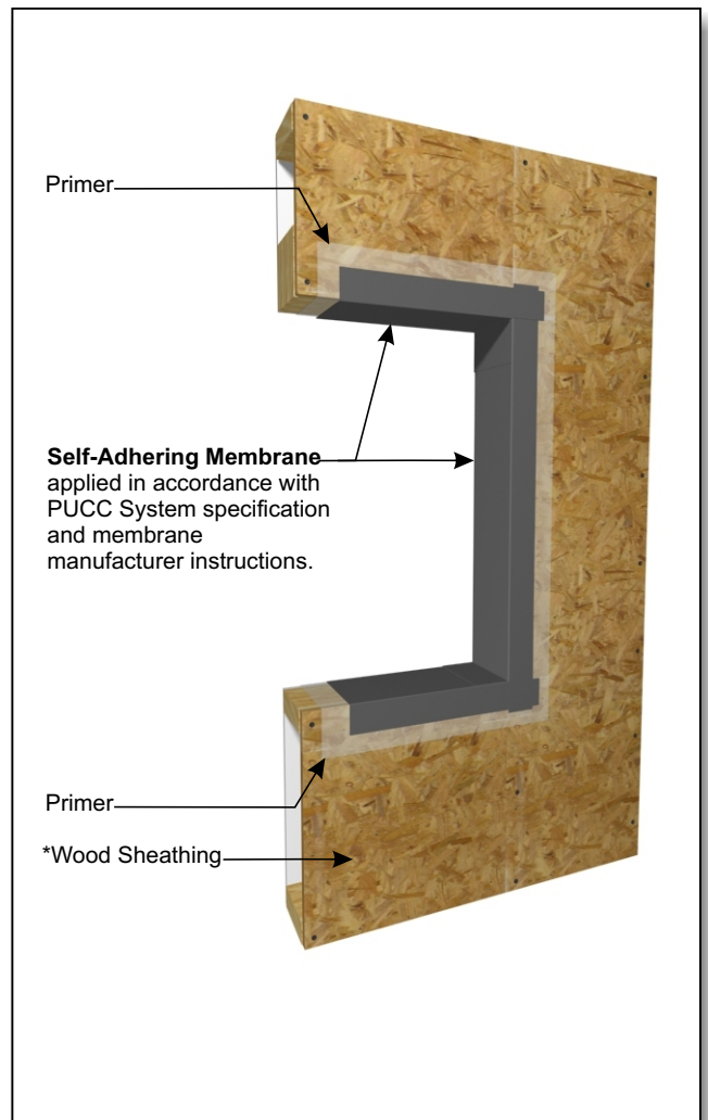
SELF ADHERING MEMBRANE ONTO WINDOW ROUGH OPENING
