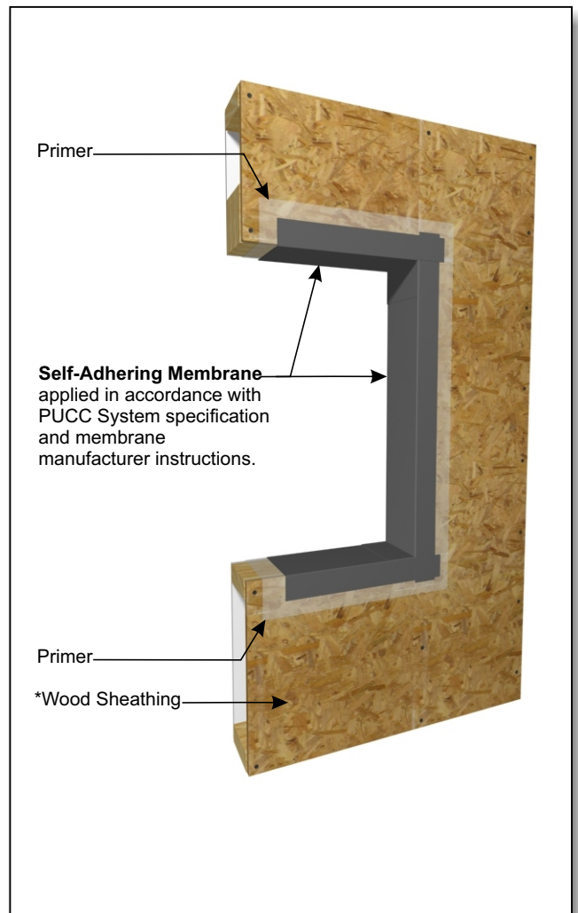
SELF ADHERING MEMBRANE ONTO WINDOW ROUGH OPENING
