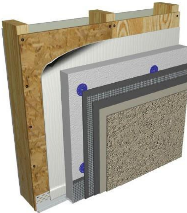
Figure 5. “InsulROCK EIFS” over modified bituminous membrane on OSB and plywood
