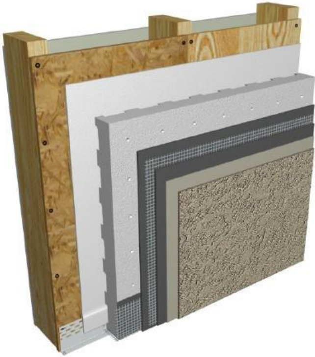
Figure 8. "PUCCS EIFS" with moisture barrier over OSB and plywood
