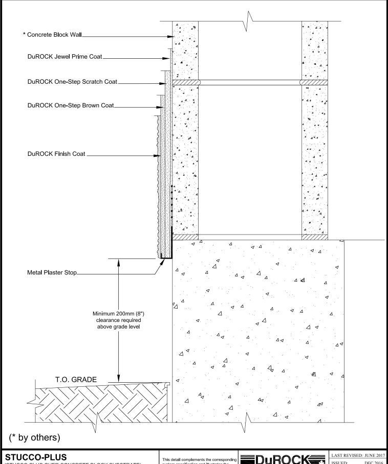
(STUCCO-PLUS OVER CONCRETE BLOCK SUBSTRATE)
