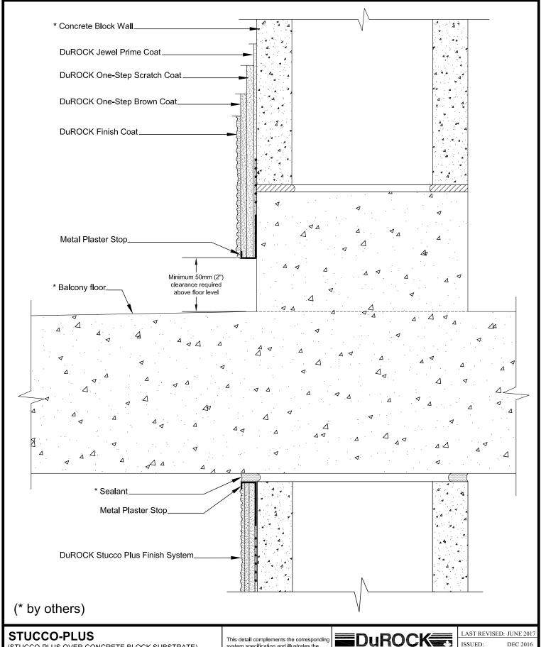
(STUCCO-PLUS OVER CONCRETE BLOCK SUBSTRATE)
