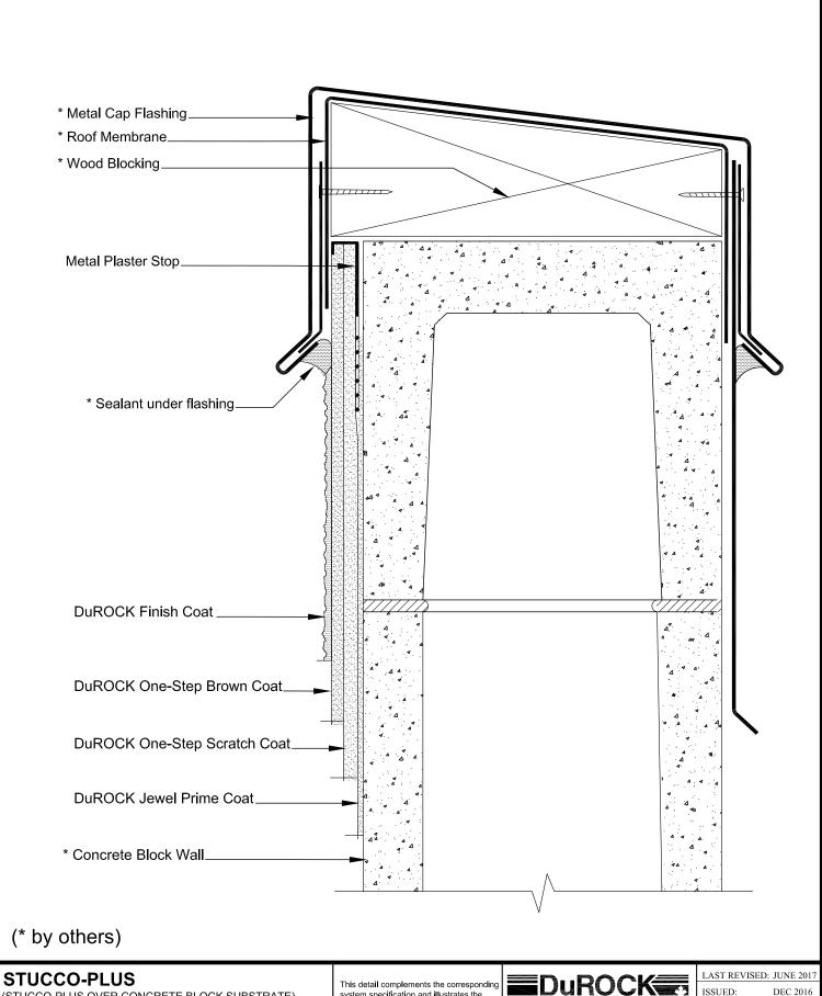
(STUCCO-PLUS OVER CONCRETE BLOCK SUBSTRATE)
