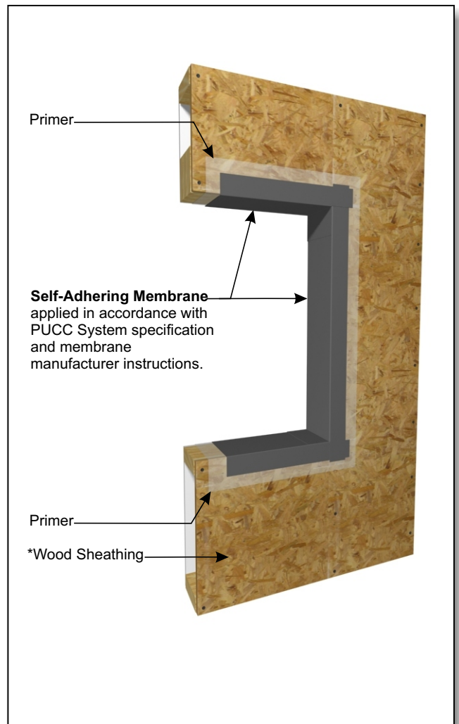
SELF ADHERING MEMBRANE ONTO WINDOW ROUGH OPENING
