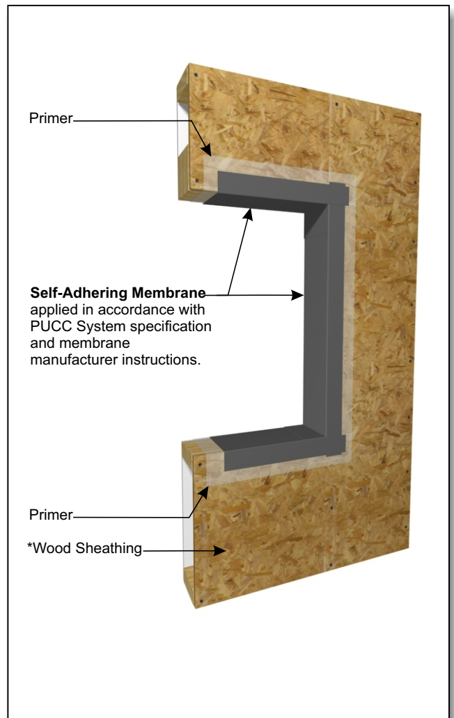
SELF ADHERING MEMBRANE ONTO WINDOW ROUGH OPENING
