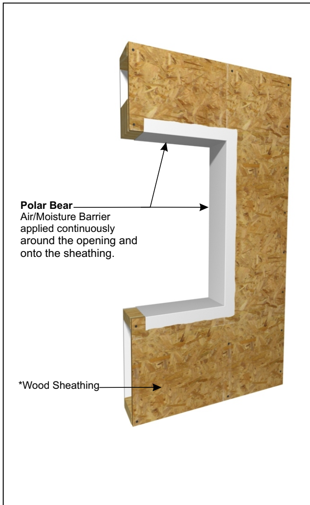
POLAR BEAR AIR/MOISTURE BARRIER ONTO WINDOW ROUGH OPENING
